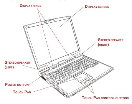
Figure 2-6 The front with the display open
